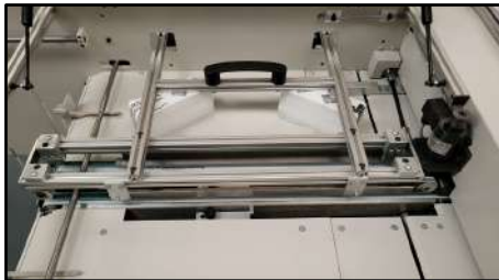
"Heart" inspired from the DocuPunch® +PLUS & EX610® to automatically adjust the set-up format with the RFID technology
