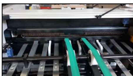
Heavy duty punching dies equipped with retractable pins
