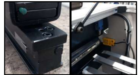
Thanks to the RFID technology into the dies, the machine configures by itself fully automatically
