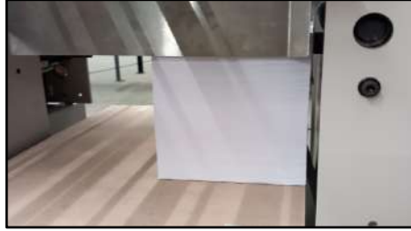
Reception with a capacity up to 13.5" (7 reams ~ 3.500 sheets (80 gsm / 20 lb bound))
