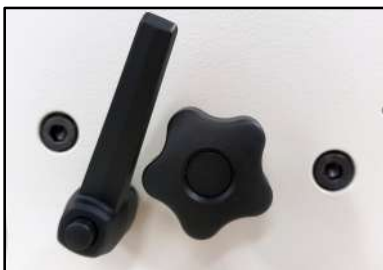
Many possible setups to adjust the parallelism of the press for a uniform closing of the Wire-O® binding
