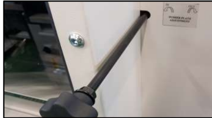
Binding is easily centred by adjusting the push plate
