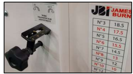
It's very easy to adjust the depth of the Wire-O® magnetic transfer bar
