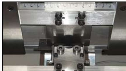
Forming device for transforming straight rods into hooks (optional)
