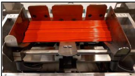
Magazine for 2.000 straight rods to feed the new module for forming and distributing hooks (optional)
